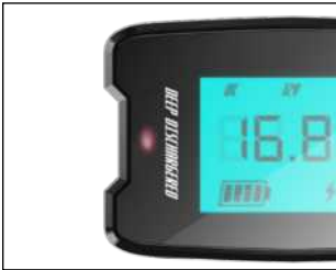
Low voltage indicator: Red LED
