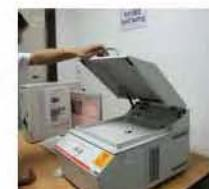
X-Ray Fluorescence Spectrometer (XRF)
